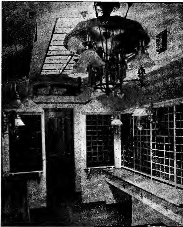
Fig. 147. INTERIOR POSTAL CAR, SHOWING LETTER CASE, END, LAMPS AND SKYLIGHT.
